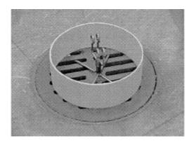
3. The adjustable clamps will accomodate 1/2– inch, 3/4–inch, and 1–inch I.D. either soft or ridgid (hard) PVC tubing. Squeezing the two tabs together that are located on the clamp–locking collar will loosen a tightened clamp.
